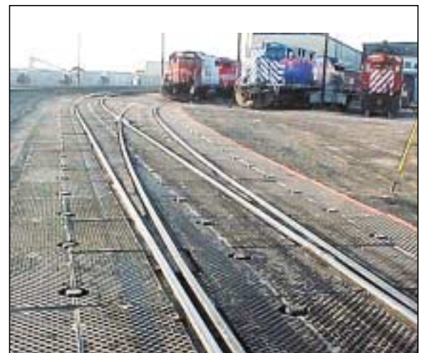
Ultra-TrackPans can be customized to accommodate switches, frogs, adjacent concrete platforms, etc.
