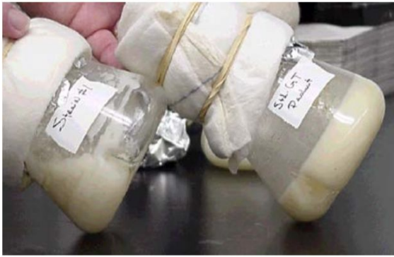
Figures 3 and 4 - Fat Degradation capabilities of two Chemtech isolates compared to a commercially available grease trap product
